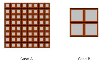
Figure 1: Packaging Overhead Versus Grainsize
