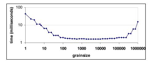
Figure 2: Wall Clock Time Versus Grainsize
