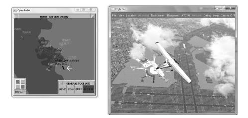
Fig. 4. Flight Gear simulator connected to modified OpenRADAR. Multiple black dots next to the white arrow in the left part of image represent the history of plane movements on virtual radar screen with KSFO airport overlay
